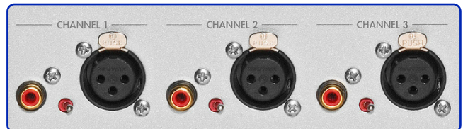
Little toggle switches on the power amp serve to select between the RCA and XLR inputs.
